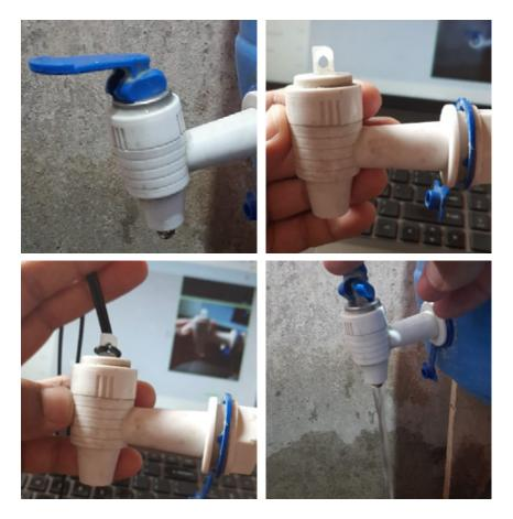
Spring loaded taps that are typically used in water filters can be fitted with a brake wire connected to a pedal
