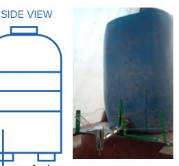
Can use any existing container: up to 20 litre system is recommended along with 2 buckets of 10 litre each that are seated on floor as back up for quick replacement.
